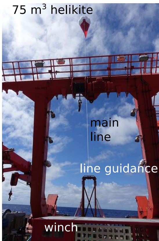
Figure 5.1.13.1 Line guidance on the aft of the working deck of R/V METEOR (left) and setup of the mini-MPCK on the 75 m 3 Helikite (right).
