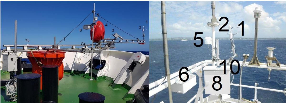
Figure 5.1.6.1 Flux instrumentation placements during M161 at the front of the vessel (left panel) and at the top of the mast (right panel): Ultra-sonic anemometer METEK uSonic-3 Scientific (1), LI-COR LI-7500 open path (2), Radiation pyrometer KT19 on sea surface (3), LI-COR Datalogger (4), temperature and humidity probe Vaisala HMT337 (5), Barometer Vaisala PTB (6), GPS receiver (7a,7b), USAT Datalogger (8), Power box (9) and GPS-mouse (10).
