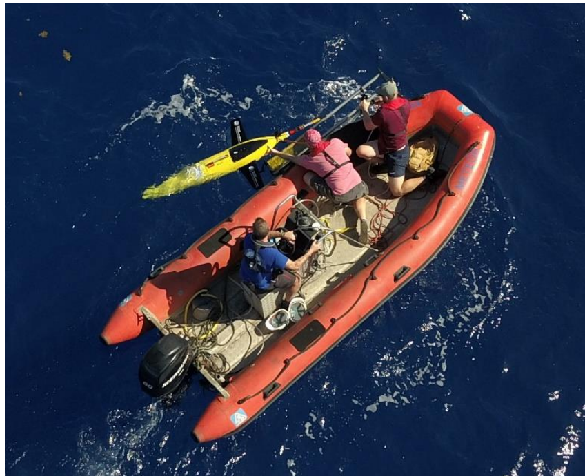
Figure 5.2.2.1 Glider deployment from the R/V METEOR's workboat as photographed by a drone.
