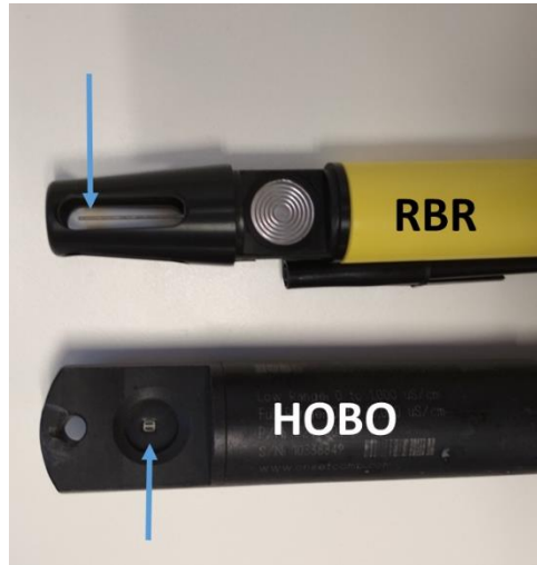
Figure 5.1.12.1. RBR and HOBO instruments with marked temperature sensors' location on each of the instruments.
