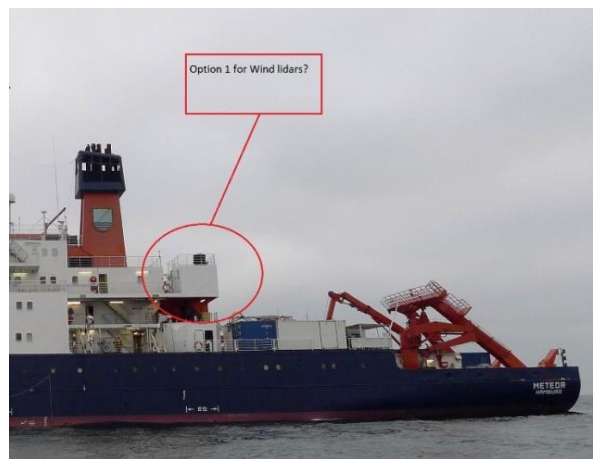
Figure 5.1.5.1 Position of the two Wind LiDARs on the Meteor. Left image shows the long-range WLS70 on the left and the short-range V2 on the right of the deck, the image orientation is towards portside. Right image shows the location of the deck above the paint storage where the LiDARs are placed.
