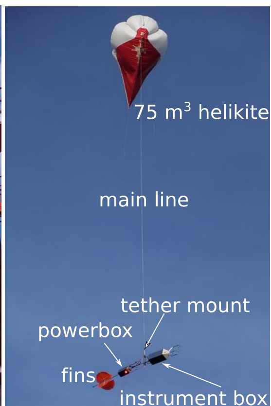
Figure 5.1.13.1 Line guidance on the aft of the working deck of R/V METEOR (left) and setup of the mini-MPCK on the 75 m 3 Helikite (right).
