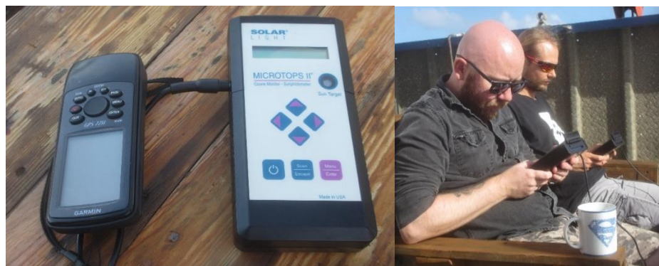
Figure 5.1.3.1 The MICROTOPS sunphotometer (left) and its handheld operation into the sun (right).
